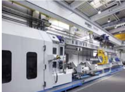
Metal spinning machine measuring 30 m in length
