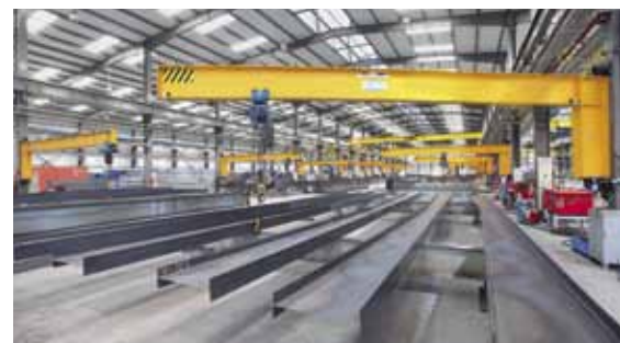
Wall-mounted slewing jibs with 8 m outreach
