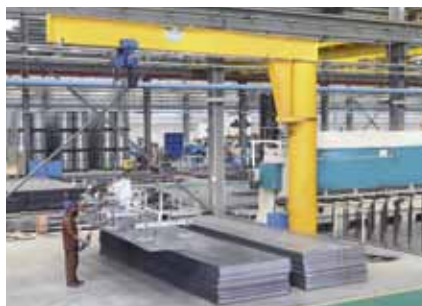
Pillar-mounted slewing jib crane with a vacuum spreader used to pick up sheet and plate steel
