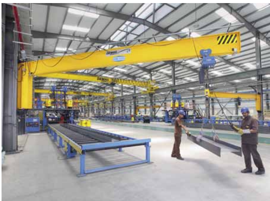
Wall-mounted jib cranes with large slewing angles
