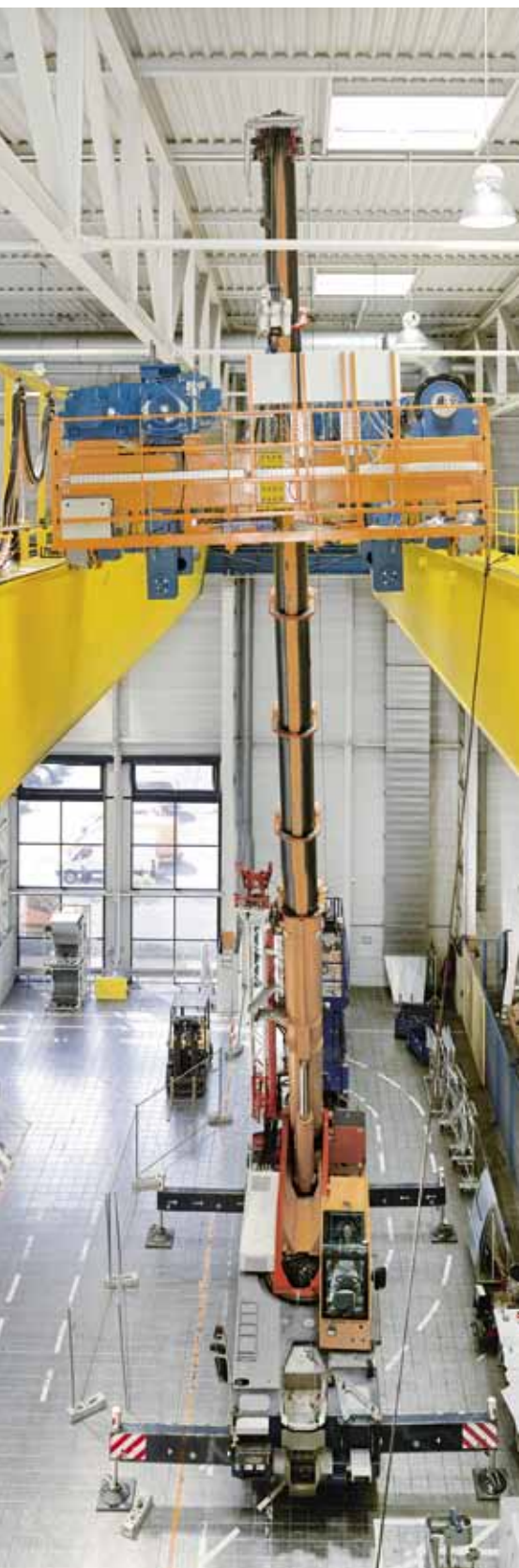
Positioning the crab on the crane girders
