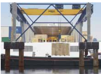
Fit for outdoor operation: ZKKE with two wire rope hoists
