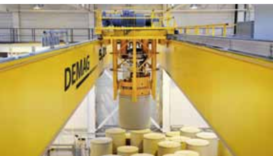
The process cranes gently transport the rolls of paper by means of vacuum lifting devices
