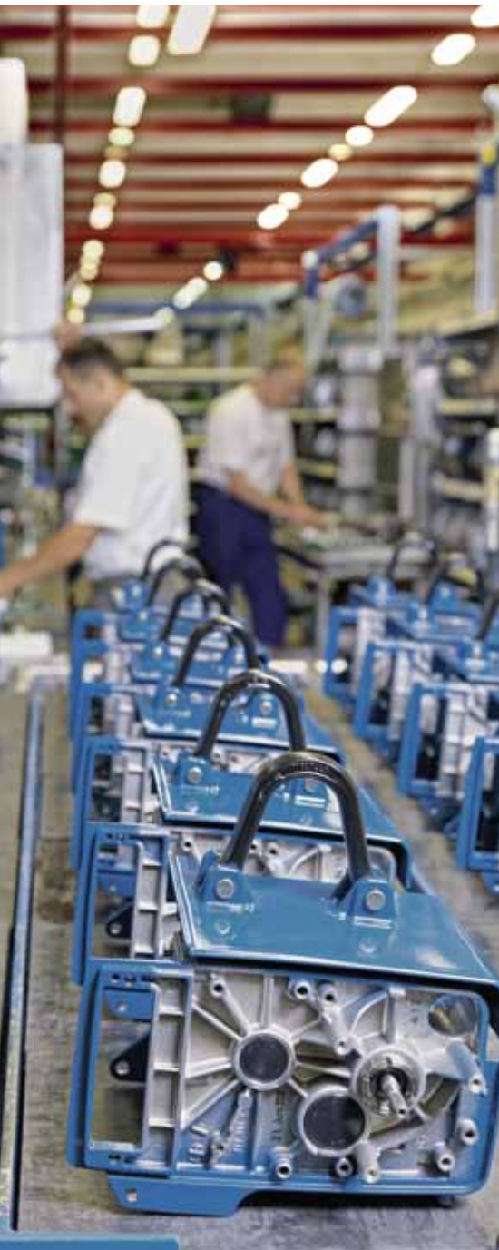
Assembly line for the DC generation of chain hoists
