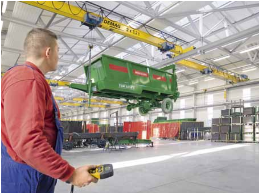
Precise control via the DRC-MP radio control system for hoists operated in tandem and as single units
