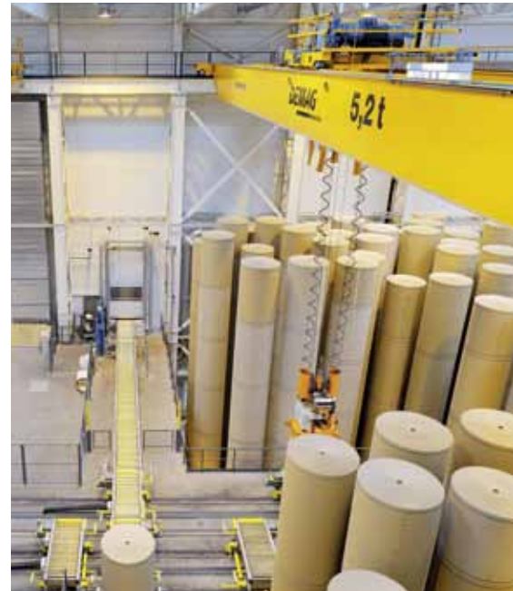
The conveyor line passes through the 90 m-long storage zones.
