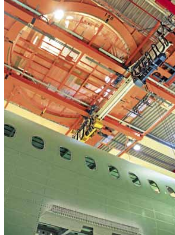
Crab equipped with turning mechanism and four hoist units
